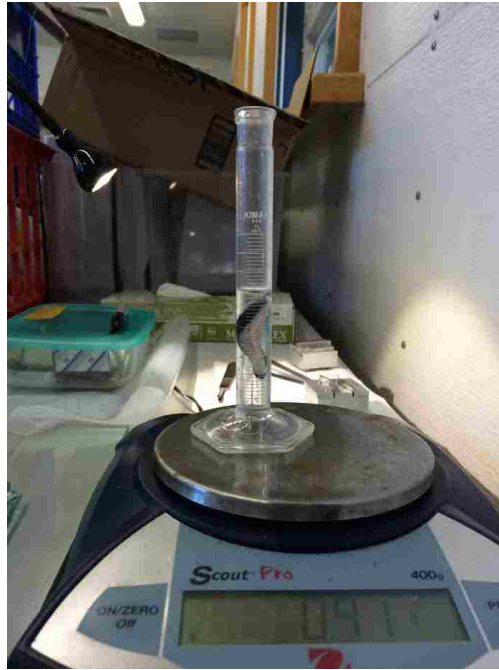
Figure 3.13: Density of skin (pictured above) measured through displacing water in a graduated cylinder, measuring the liquid displacement and change in mass.
